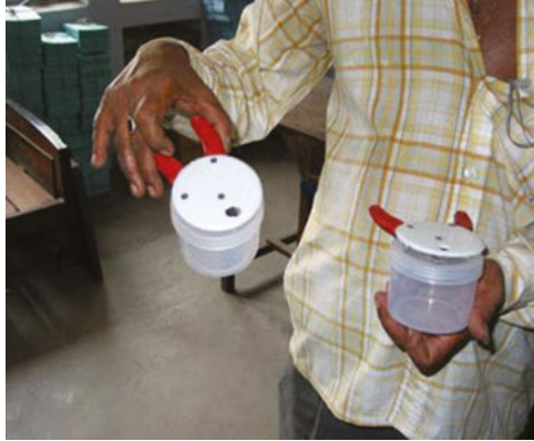
Figure 6.1 Needle cutter that was locally produced in West Bengal, India, for the Japanese encephalitis immunization campaign (picture by Julie Jacobson).
